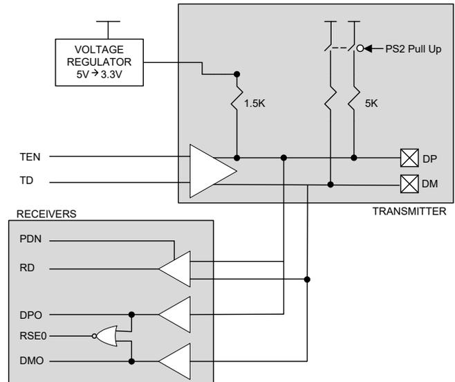
At the enCoRe V system level, the full-speed USB system resource interfaces to the rest of the enCoRe V by way of the M8C's register access instructions and to the outside world by way of the two USB pins. The SIE supports nine endpoints including a bidirectional control endpoint (endpoint 0) and eight unidirectional data endpoints (endpoints 1 to 8). The unidirectional data endpoints are individually configurable as either IN or OUT.
