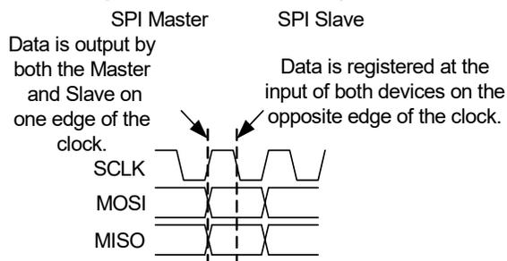
A device can be a master or slave. A master outputs clock and data to the slave device and inputs slave data. A slave device inputs clock and data from the master device and outputs data for input to the master. Together, the master and slave are essentially a circular Shift register, where the master generates the clocking and initiates data transfers.
