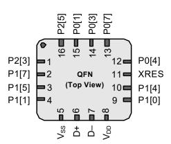
Figure 6. CY7C64315/CY7C64316 16-pin enCoRe V USB Device
