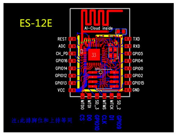
And here is the schematic for the ESP-12F. Note that the ESP-12E and ESP-12F are said to be identical except for the antenna (which is better on the ESP-12F).
